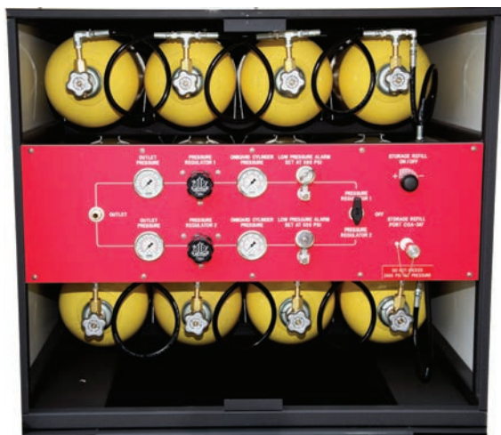
Long Duration Air Storage Hazardous Response Trailers
