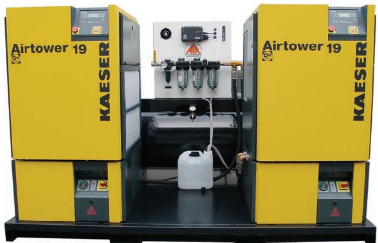
Dual Compressors with Auto Sequencing
