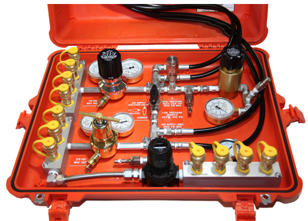
MACK-3™ with optional MACK-3FA fill regulator to fill high pressure cylinders
